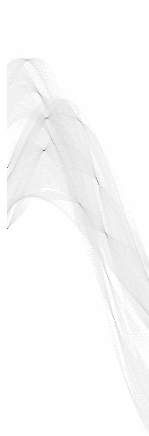
Figure 7. Hough transform – Hough's space of the input image on Figure 1, (x-axis representing  $\varphi$  and y-axis representing  $r$ ).
