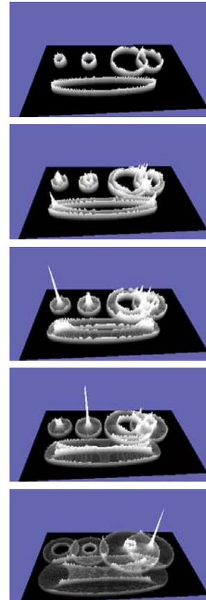
Figure 13. Hough's space for increasing radius (descending) in 3D. (x-axis representing a, y-axis b and z-axis representing intensity).
