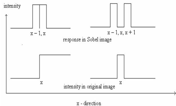
Figure 4. Sobel edge detection operator, reconstruction of original line objects (in contrast to finding the outlines)
