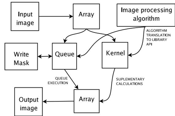
Figure 1: Overall model of computation using proposed library architecture. Image data is stored inside *Array* objects. Image processing algorithm is implemented by *Queue* and/or *Kernel* computation engine
