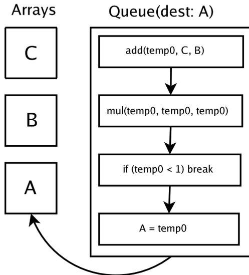
Figure 2: Example of a *Queue* instance with conditional instruction execution. The *Queue* type can be imagined as a container for a set of operations. Executing a *Queue* means executing serially all the operations inside, beginning from the first one added.
