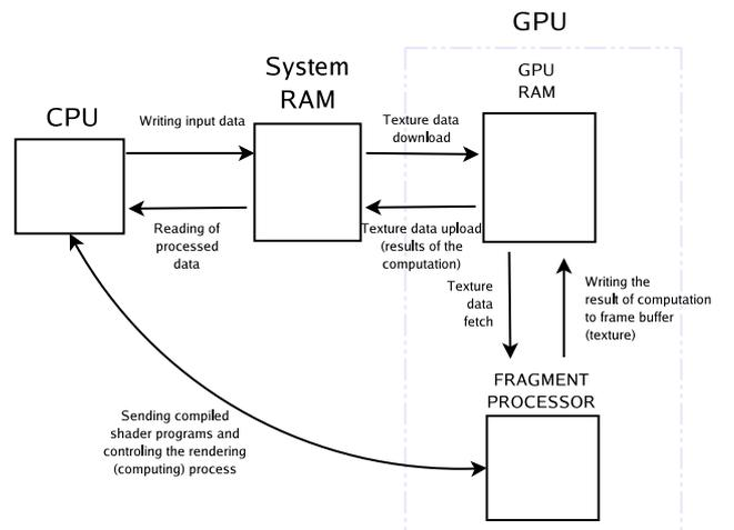
Figure 4: CPU-GPU interaction in computation.
