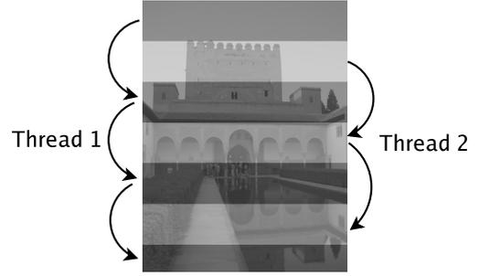
Figure 3: *Queue* execution on multicore CPU. Data is divided into small chunks. Each chunk is assigned to execution *Thread*. On this example *Thread 1* is processing chunks 0, 2, 4, 6 and *Thread 2* the remainder, chunks 1, 3 and 5.
