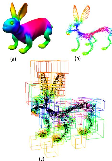
Figure 7: (a) mesh with SDF values, (b) projected points resembling medial axis, (c) octree nodes containing the average SDF values.
