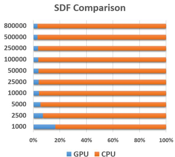
Figure 10: Benefits of GPU implementation with varying level of detail. Comparison was performed on model of Stanford Dragon.
