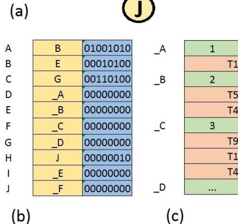
Figure 5: Octree topology on an example. (a) octree structure, (b) 1st array with octree nodes, (c) 2nd array with leaf data.
