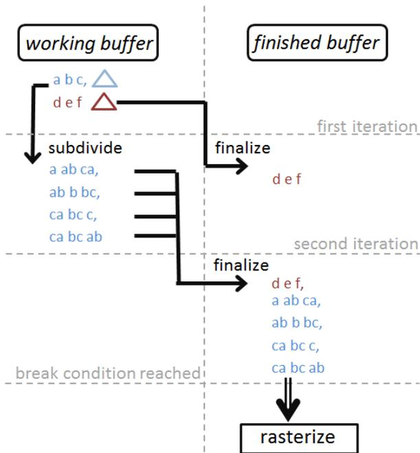
Figure 6: The tessellation loop iterates until the working buffer is empty or maximum iterations is reached.
