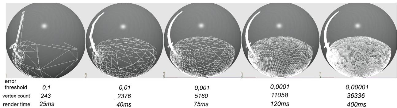
Figure 8: Adaptive tessellation with different error threshold values.
