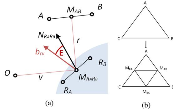
Figure 5: (a) The reflection error  $E$ . (b) The subdivision rule used to tessellate a triangle.
