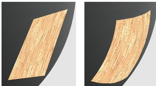
Figure 1: *Left:* Erroneous reflection of a square. Its sides are linear interpolations between the corners' reflections. *Right:* Correct reflection after sufficient tessellation of the square.
