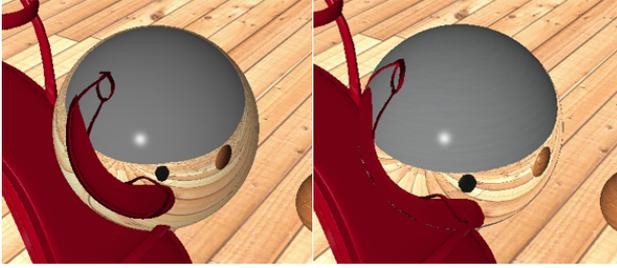
Figure 2: *Left*: Approximate reflection using Environment Mapping with errors. *Right*: Accurate reflection.
