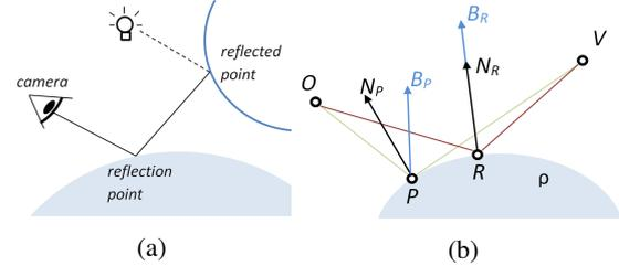
Figure 3: (a) Reflections are found by tracing light paths. (b) The relation between the viewpoint  $O$ , the world vertex  $V$  and a point  $P$  on the reflector surface  $\rho$ . The reflection point  $R$  is such that their bisector vector  $B_R$  and the surface normal  $N_R$  coincide.
