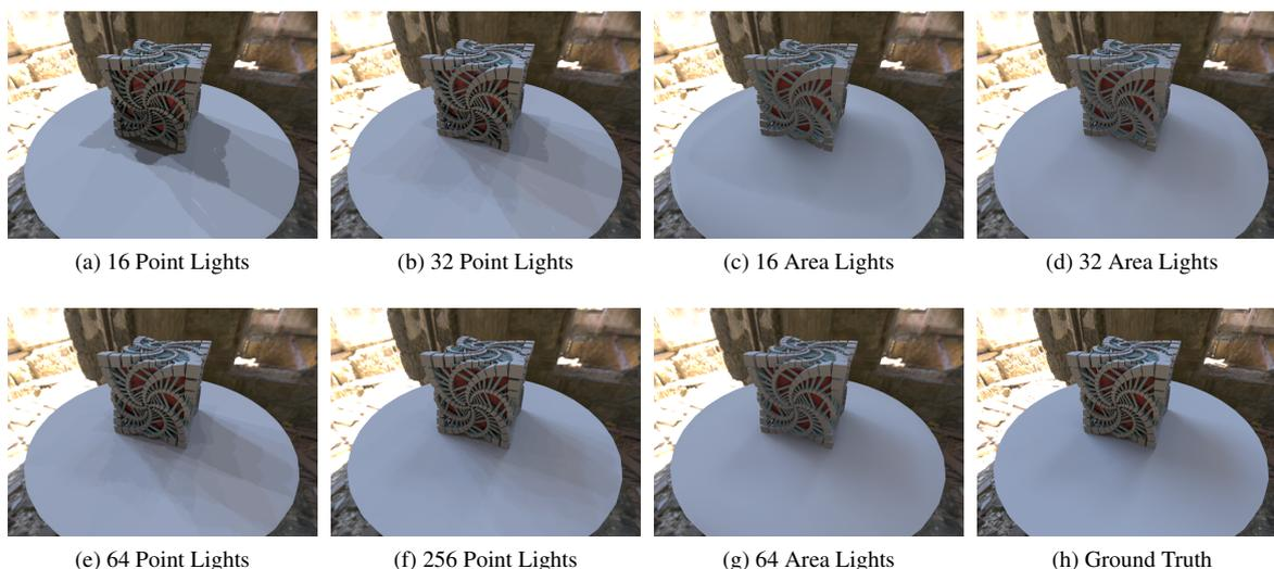
Figure 2: Scene illuminated by different amounts and types of light sources, extracted from the light probe. The ground truth (h) was rendered using a path tracer considering direct illumination only.
