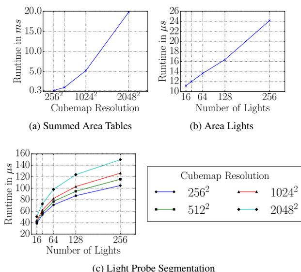
Figure 3: Runtime for generating area lights on the GPU. (a) shows the runtime for computing the SATs from the raw light probe. (c) shows the runtime for the median cut algorithm, and (b) show the runtime required to retrieve the parameters of the area lights from the final regions.
