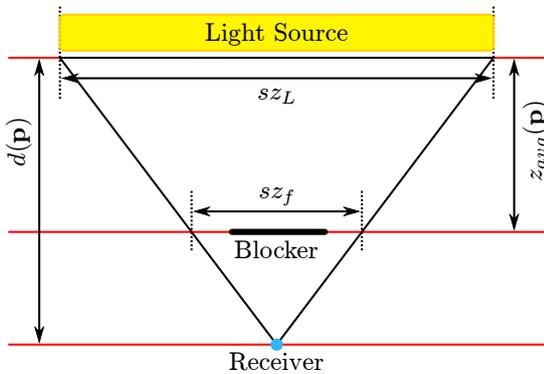
Figure 1: Illustration of the relation between fragment depth  $d(\mathbf{p})$ , average blocker depth  $z_{avg}(\mathbf{p})$ , area light size  $sz_L$  and filter size  $sz_f$ .
