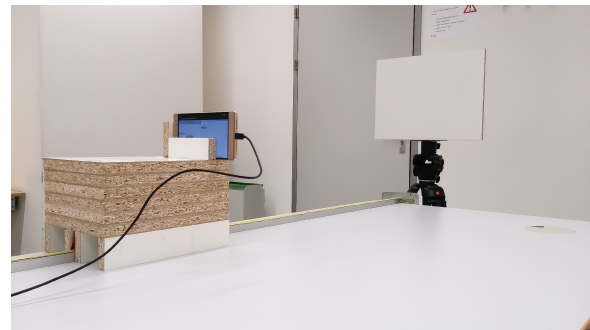
Figure 3: Images of the setups for the two different sensors, consisting of a fixed, wooden plane and a moving construct for the sensor
