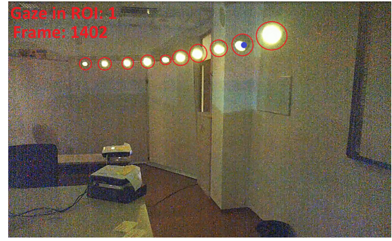
Figure 5: Automatically evaluated frame from the eye-tracker. Tracked ROIs are in red circles, gaze point in the current frame is a blue dot. Evaluation module stated that a fixation in ROI number 1 is present (numbered from 0, beginning from the right-most ROI).
