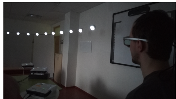
Figure 2: Participant ready to start an experiment captured along with the complete scene setup with desired projection on the ROIs. The eye tracker is mounted to a PC with running data acquisition module.
