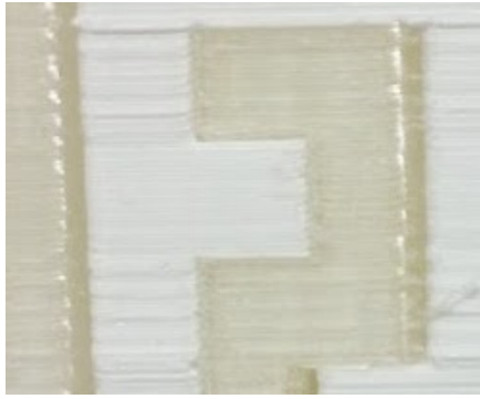
Figure 14: Vertical delamination of the PLA and PVA filaments.
