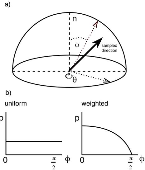
Figure 3: **a)** Illustration of hemisphere sampling. **b)** Uniform versus cosine weighted probability density function of upper hemisphere sampling.
