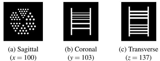
Figure 9: Slices of the Derenzo Phantom
