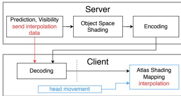
Figure 2: SAS pipeline overview, with modified stages highlighted red, the blue sections represent a decoupled part from the server to perform frame-rate upsampling
