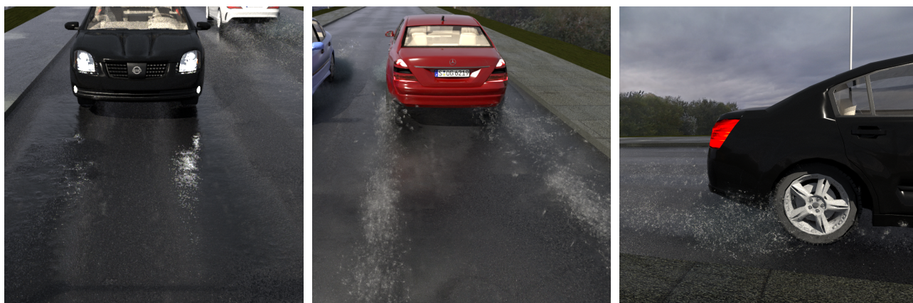
Figure 1: Images of the wet road simulation acquired via ray-tracing. The figure on the left displays a wet road flooded with shallow puddles. The car's headlights reflect on the puddle surface. Splashes of water projected from the tires can be seen in the central figure. The last figure shows a close-up of the splash.
