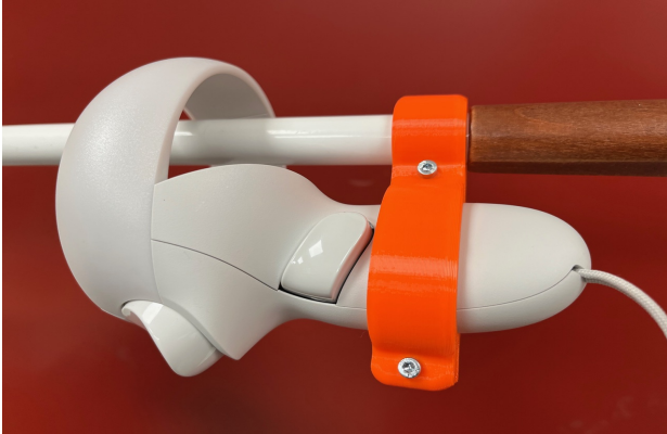
Figure 3: Implementation of the real world cane with a controller coupled via a 3D-printed holder, mounted right at the end of the cane next to the handle
