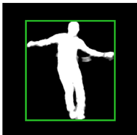
Figure 2: Segmentation mask with overlaid rectangle, which coordinates were calculated based on the edges of mask's contour. As a result, an optimal bounding box around the entire human body is found.
