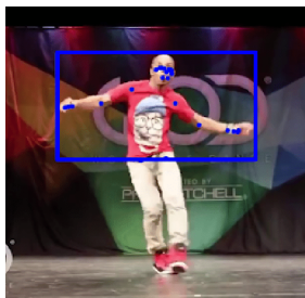
Figure 3: Bounding box, derived from the segmentation mask, cropped based on the y-coordinate of hips pose landmark.
