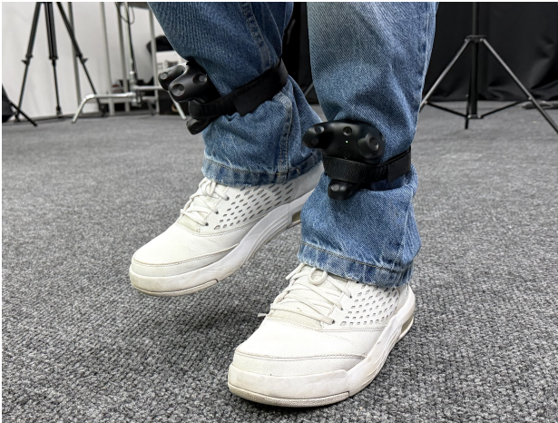
Figure 2: HTC Vive trackers attached to users' legs
