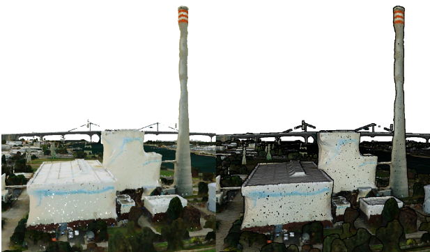
Figure 7: Without EDL (left) and with EDL applied (right), which enhances depth perception by highlighting depth discontinuities.
