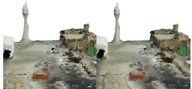
Figure 6: Naive rasterization (left) and the three-pass blending approach (right), which blends neighboring points at similar depths, creating smoother surfaces.
