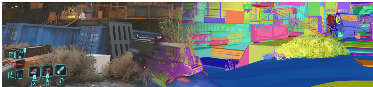
Figure 1: A ray-traced scene from Cyberpunk 2077 (left) and its underlying ray tracing acceleration structure (right) as visualized by NVIDIA Nsight Graphics [29] frame capture tool.
