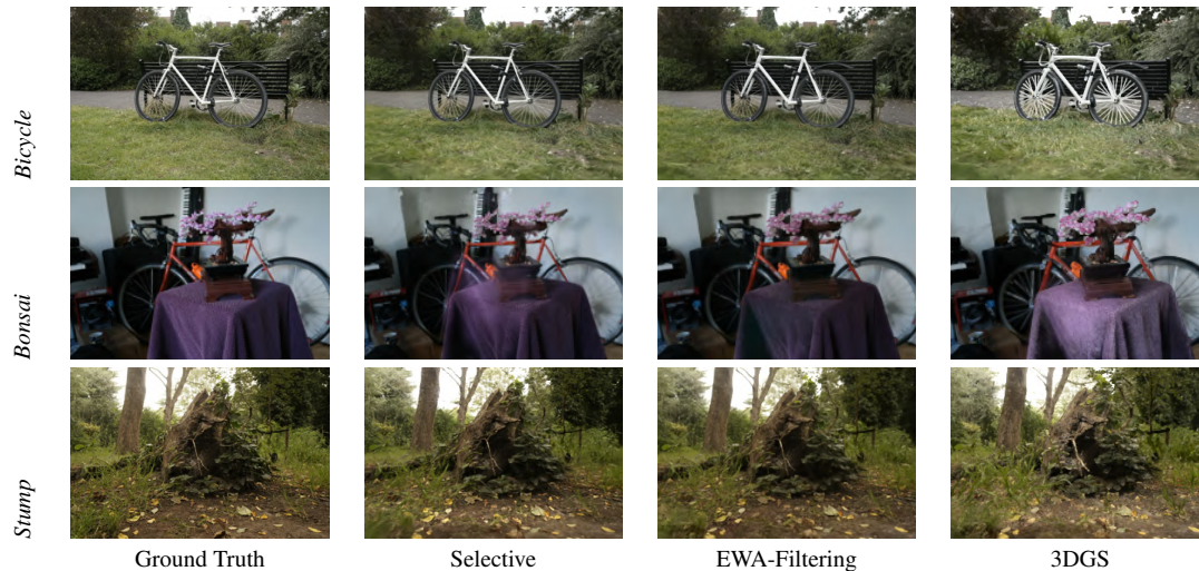
Figure 8: Qualitative comparison of the ground truth images and the renderings at one-quarter resolution from the test set of different scenes. Selective rendering (2nd column) effectively reduces aliasing errors, similar to EWA-Filtering (3rd column), which are present in renderings from 3DGS (4th column), where thin structures are rendered too thick and too bright.
